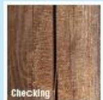
**Checking, or cracks, occur across or through the growth rings as they release moisture.** This is a natural process and is common to all wood species. Checking is not a defect in the wood; it does not diminish the quality, durability, safety, or the structural integrity. Instead, it is considered a part of the log's rustic natural look and adds to the uniqueness of each piece.
